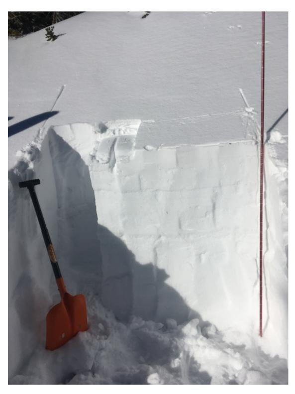
This pit was dug near Maid of the Mist in Hyalite. It produced unstable test results on a thin weak layer 10" down from the surface. ECTP22 @22cm. SE slope at 9700'. HS 110cm. Photo: M. Zia
