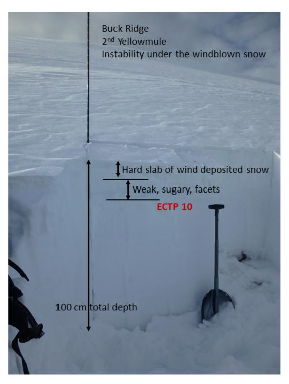
Our snowpit showed instability in the small, sugary facets that are underneath a hard slab of wind blown snow. An avalanche was triggered around the corner from this snowpit around the same time we were digging! Photo: GNFAC
