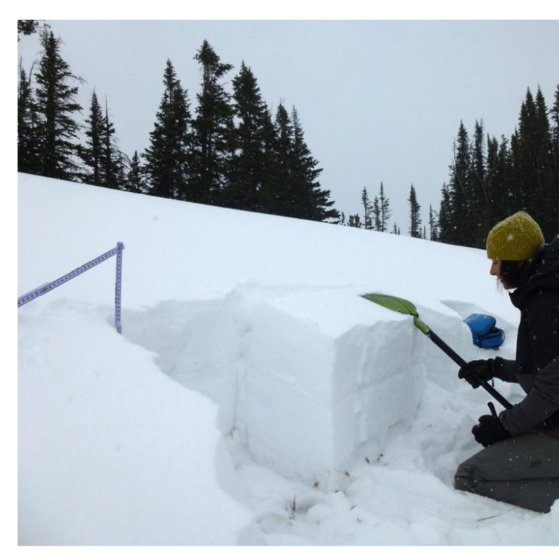
**Stable and weak.** Dug a pit on an E aspect (HS 69cm) near Pika Point. Pit composition was fairly uniform, with multiple layers of different sized facets/rounding facets. Had a clean break, CT13, Q2 on facets beneath the Thanksgiving crust, though did not propagate (ETCN21). Found a 2 inch layer of near-surface facets, which will likely cause some problems with more precipitation on the way later in the week. Photo: GNFAC
